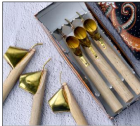
Görsel 18. Geleneksel Tjanting Batik mumlama kepeçeleri, https://kraftkolour.net.au/collections/batik-tools/products/authentic-indonesian-tjanting-set-of-3-fine-medium-large-spout (Erişim tarihi 25.02.2023)
